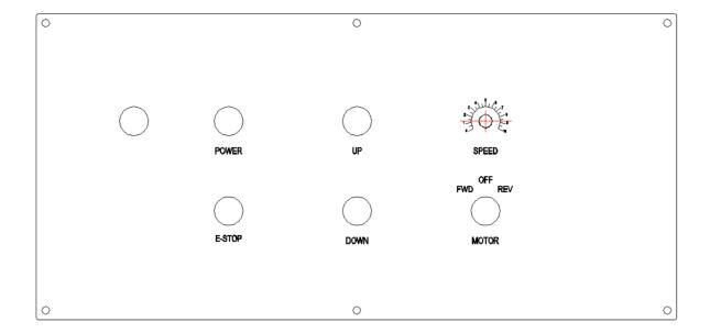
Swtich the main power on. Turn keyed switch on, then the machine is ready to run. The motor switch is used to control the start, stop and direction. The mixer head speed can be
